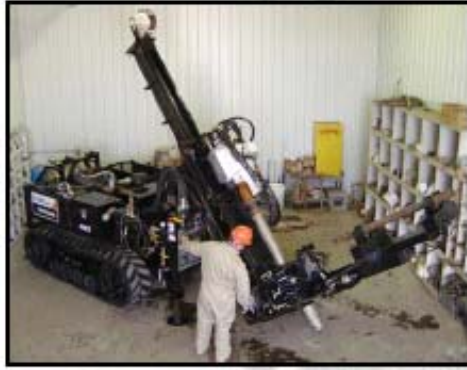
Photograph 1 : Minisonic drill rig for low head room, tight access projects.
