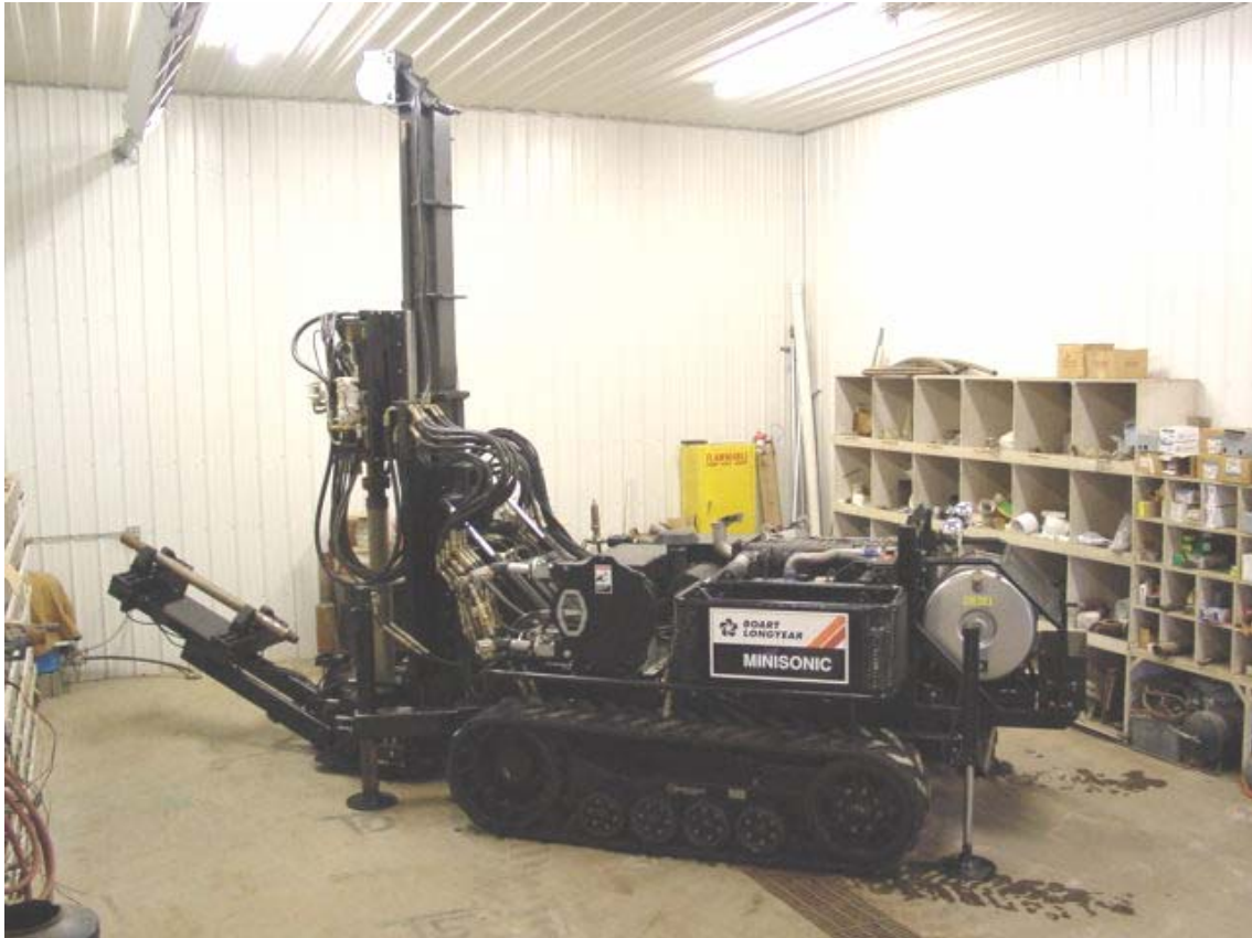
Figure 5. Track mounted "mini sonic" drill rig for low headroom applications.
